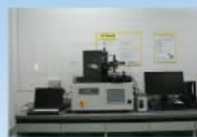
Friction & Wear Tester (Tribogear)
